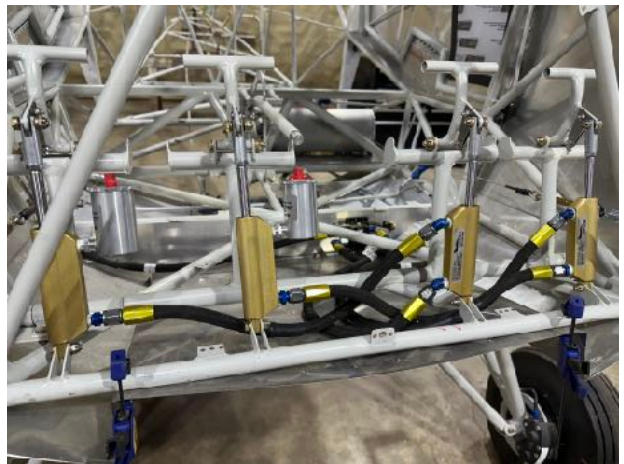
Brake System Completed and Parking Brake Installed
