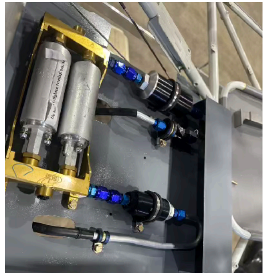
Fuel System Completed to Firewall
