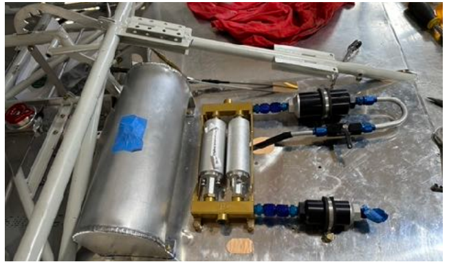
Header Tank and fuel pumps
