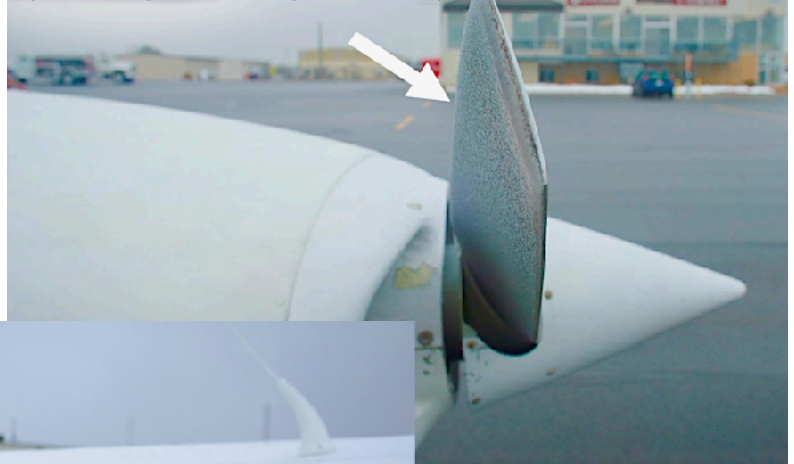
Freezing Drizzle Accumulation (Wind Blowing From Left To Right On The Ramp)
