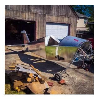
Other features include differential cable brakes, modified full swivel Scott tail wheel, a standard canopy with bonded sides (no rivets), and an exterior canopy handle to open it.
