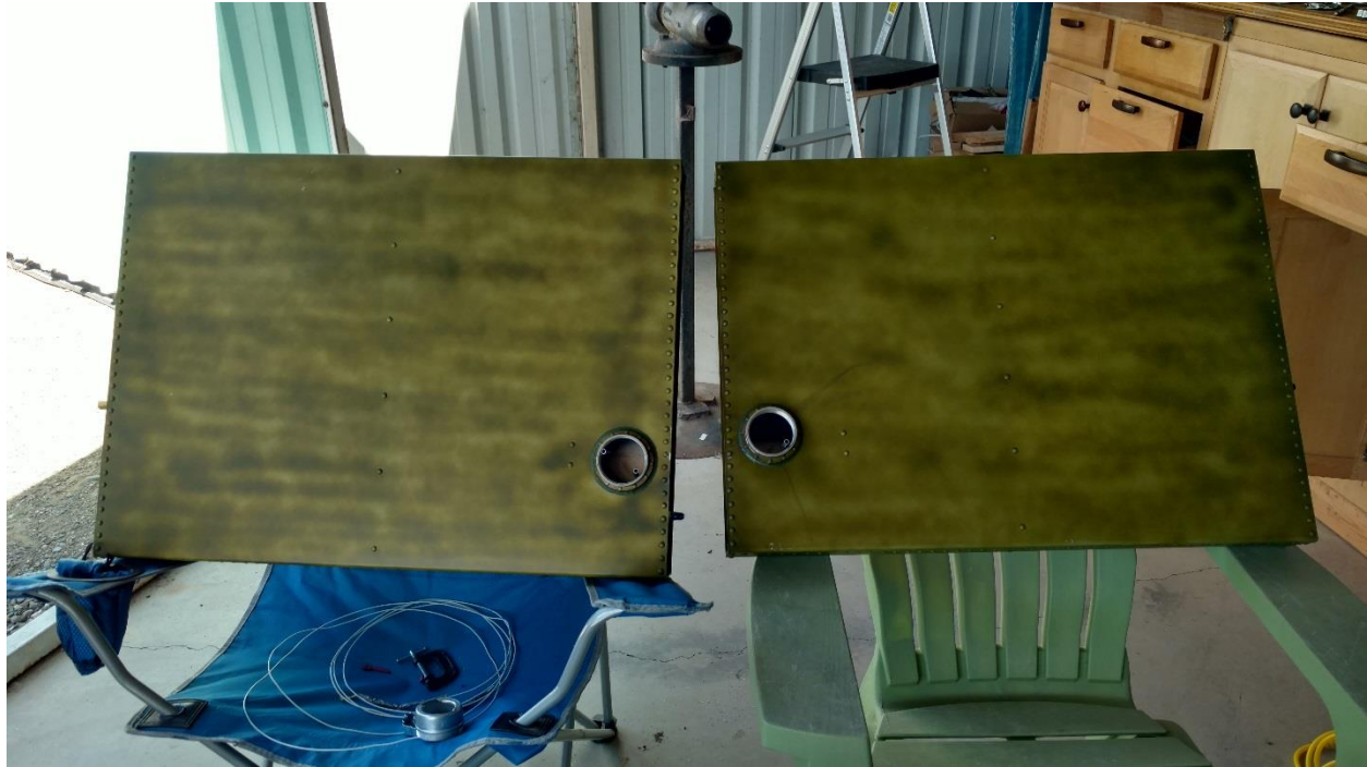
Primered tanks ready to install.
