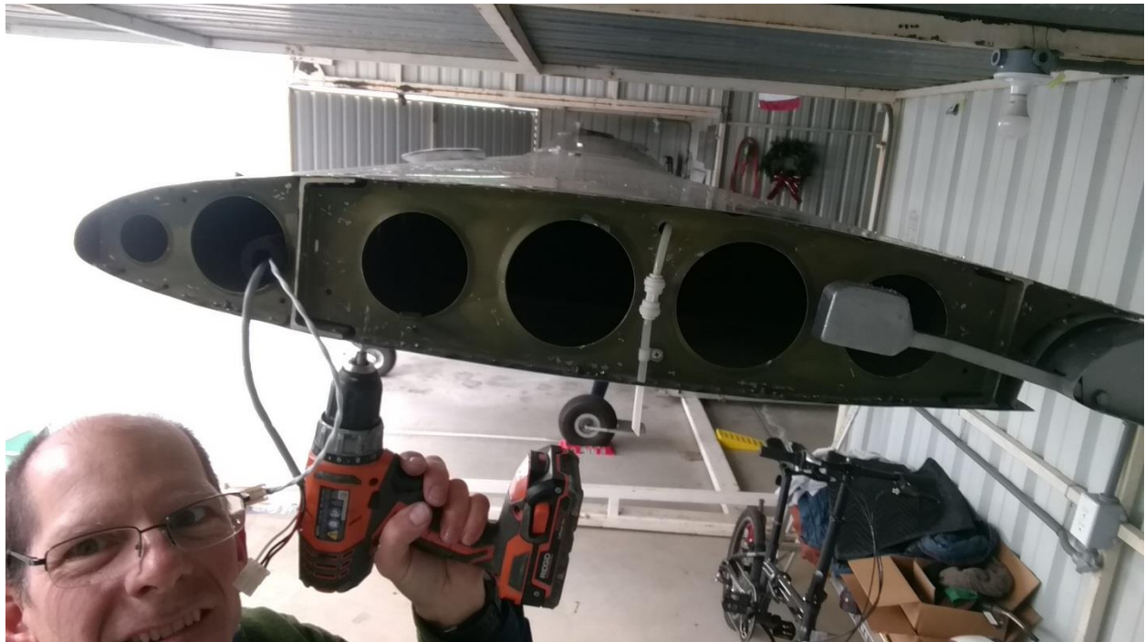
Removing the end wing rib to expose fuel tank bay.
