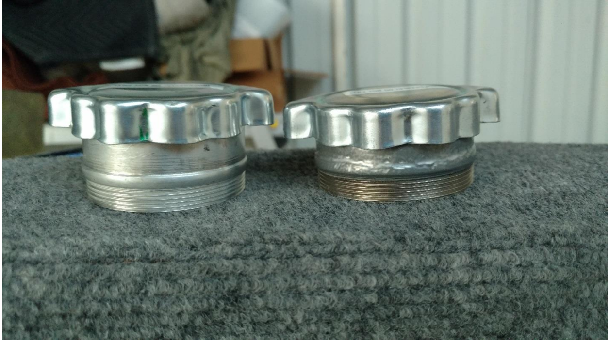
Unmodified filler neck on left, modified on right.
