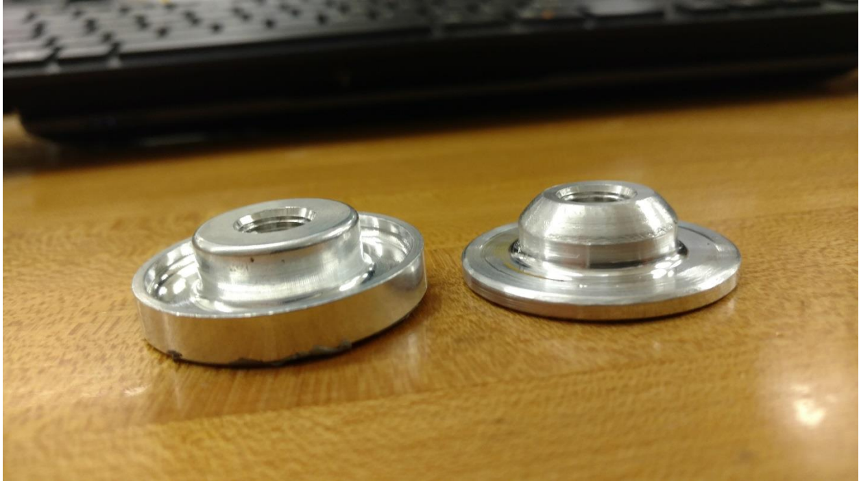
Welding flange on the right for tank vent has been modified for use with rivets.
