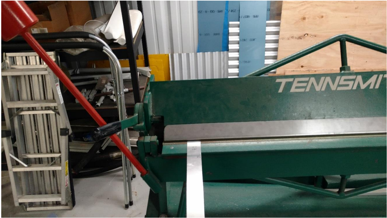
Practicing bending a test piece in the sheet metal brake.
