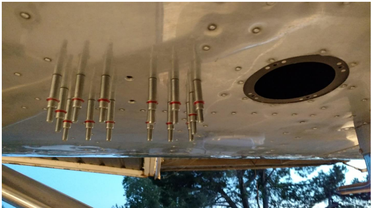
Wing skin doubler held in place with clekos ready to rivet.
