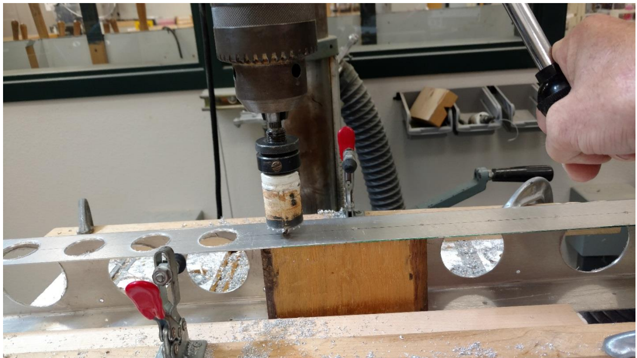
32 lightening holes were made in the channels to save weight.
