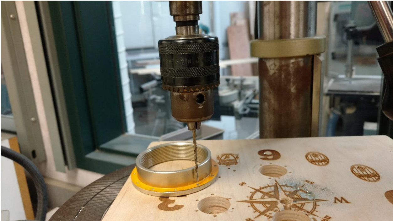
Drilling rivet holes in the filler neck flange. Note the yellow vinyl sticker showing hole locations.
