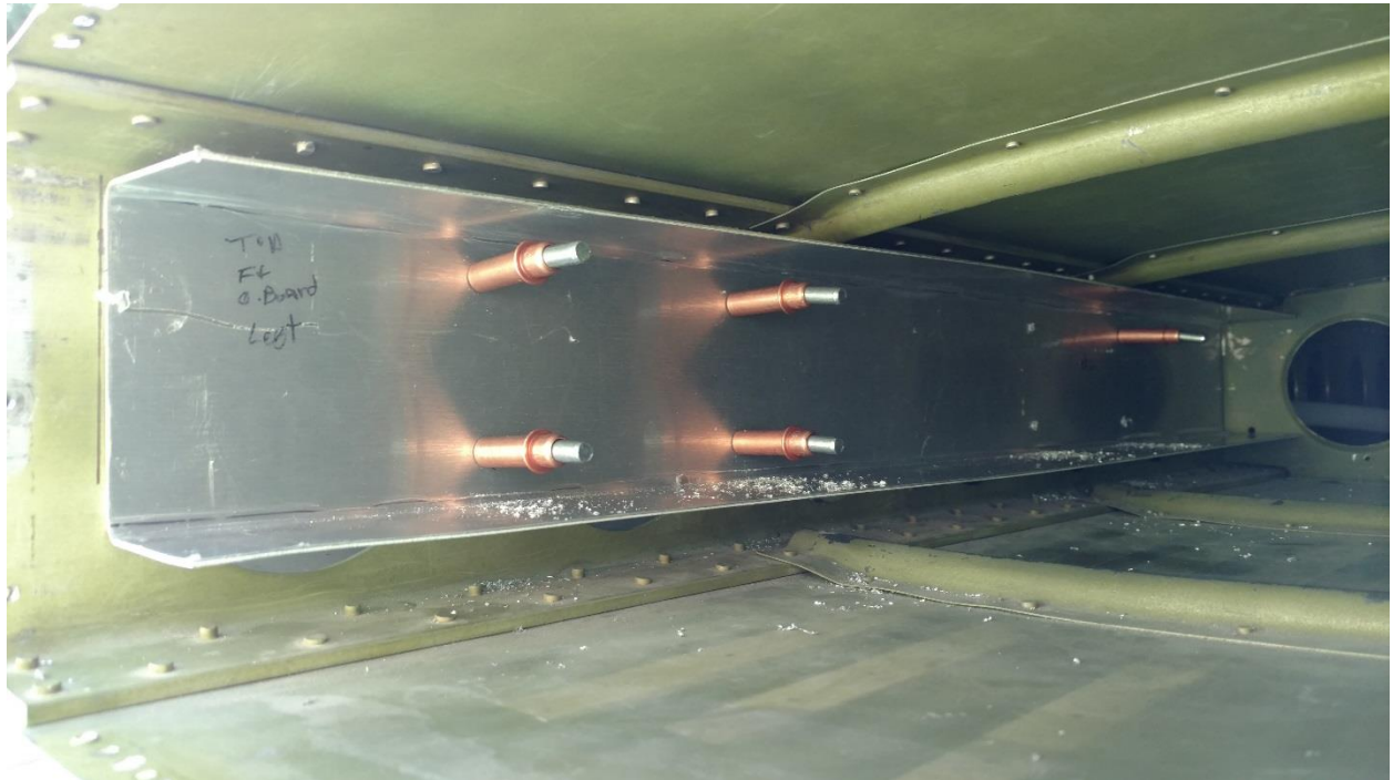
Channel that holds tanks temporarily held to the wing spar with clekos.
