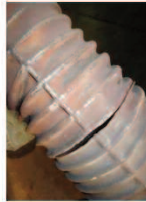
Figure 1. Photographs of a cracked muffler and exhaust deposits in the muffler shroud.
