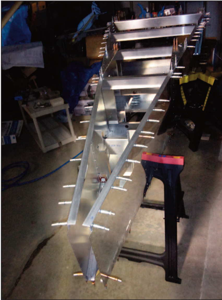
Aft fuselage box of Joe Kirik's Waiex framed up, Y tailpost goes on next.
