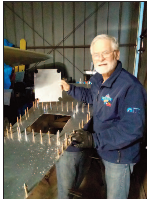
What can be more satisfying than cutting a big honkin' hole in a fuselage skin for an access panel?
