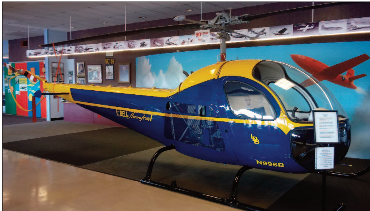
Bell Aircraft President Larry Bell ordered design and production of the model 47H-1 because he disliked the open center frame and tail boom of the standard Model 47. It incorporated a deluxe upholstered cabin with seating for three, a semi-monocoque tail boom, contoured 35-gallon fuel tanks and an enclosed baggage compartment. Bell built 33 of these in 1955-56. This example was Larry Bell's personal helicopter which our own Dave James restored.
