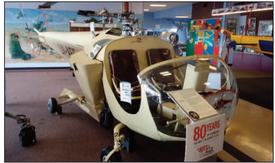
In 1947 Bell built 13 helicopters equipped with insecticide dispensing equipment. They were sent to Argentina to help control a severe locust infestation. It was believed that the unique rotor downwash characteristics swirled the dusting material over and under the plant leaves in a very precise and efficient manner.
