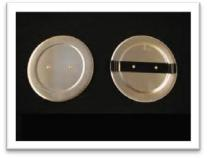
This is an example of the "slide in place" inspection plates found on fabric covered planes. These provide no structural value, but the hole in the fabric must have a reinforcing ring installed to control tearing.
