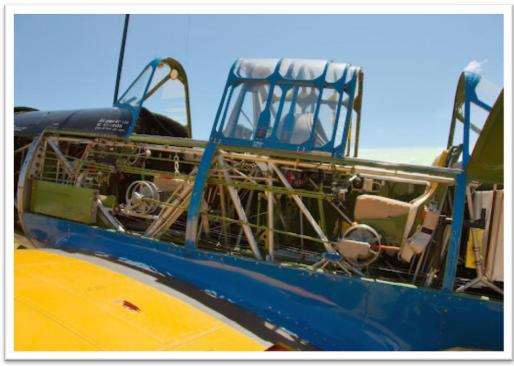
The military wanted planes designed for ease of inspection. This BT-13 provided for the entire aluminum side skins to be quickly removed. However, the steel tube fuselage provides all the fuselage strength and the side panels just act as covers for streamlining.
