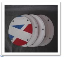
This is an example of the typical circular inspection panel covers found on Pipers or Cessnas. Usually these are held in place with sheet metal screws and are not intended to be part of the structural design
