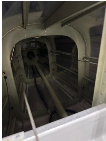
Looking rearward from cockpit to inspect the elevator pushrod assembly.
