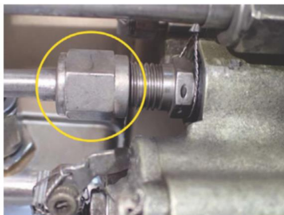
Figure. Loose B-nut at the fuel control unit of the accident engine (SOURCE: ROLLS-ROYCE ENGINES).
