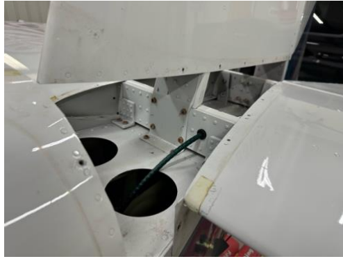
Removing the empennage cover shows the horizontal and vertical fin structure along with the elevator pushrod.
