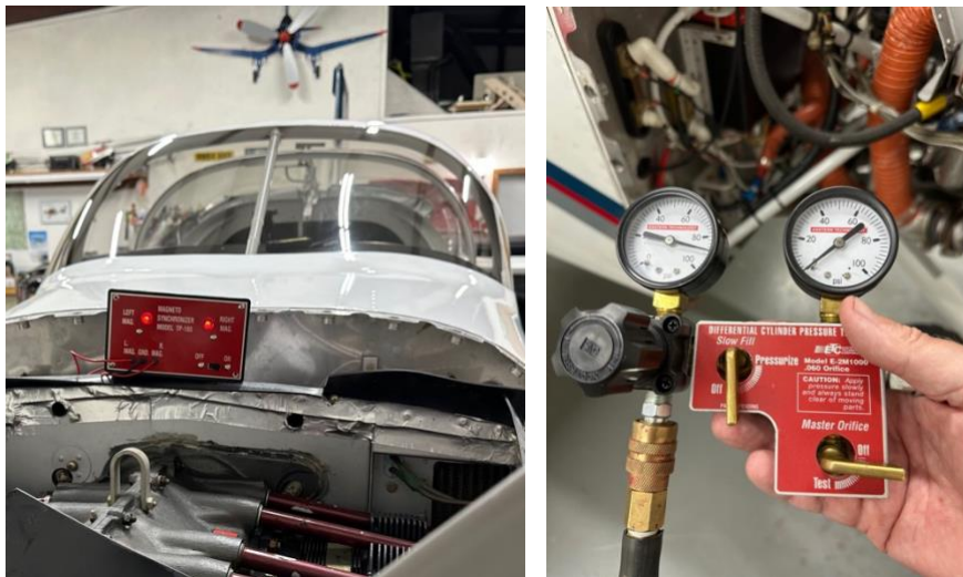
Engine Timing and Cylinder Compression Require special tools and a second pair of hands.
