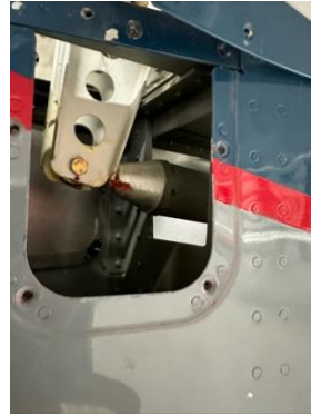
Removing the empennage cover shows the horizontal and vertical fin structure along with the elevator pushrod.
