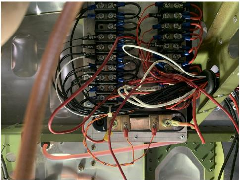
The Heart of the Failures. Note melted wires, displaced grommet, wire laying on sheet metal edges, and daisy chained buses
