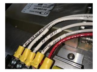
**Routing in place harness construction -** Building harnesses in place can be frustrating. Use the rubber band clamp shown in the picture below to easily control wires as you add, subtract, and re-route wires in the harness in aircraft. Use the clamps the same as a wire tie to hold bundles together and in place. Go back later and add wire ties to pull the harnesses in tight.
