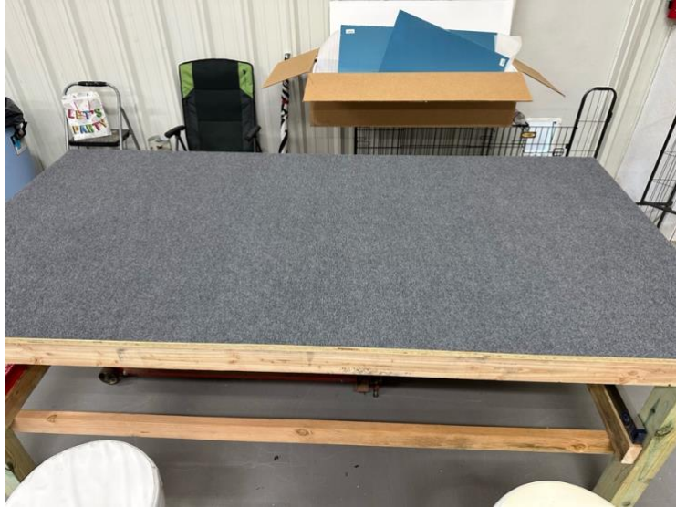
Custom Fabricated 8x4' Workbench including carpeted surface to minimize scratching of parts during handling and assembly.
