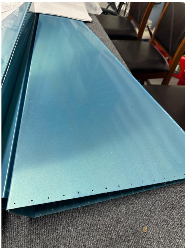
Kit parts come pre-bent with rivet holes pre-drilled.
