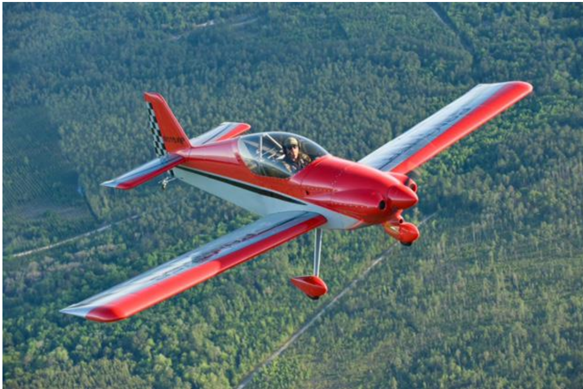
SPA Panther is a single seat Light Sport airplane with folding wings.
