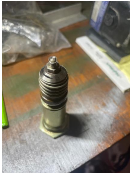
Figure: Changing the Vernatherm to fix high oil temperature.
