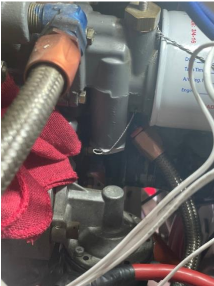
Figure: Changing the Vernatherm to fix high oil temperature.
