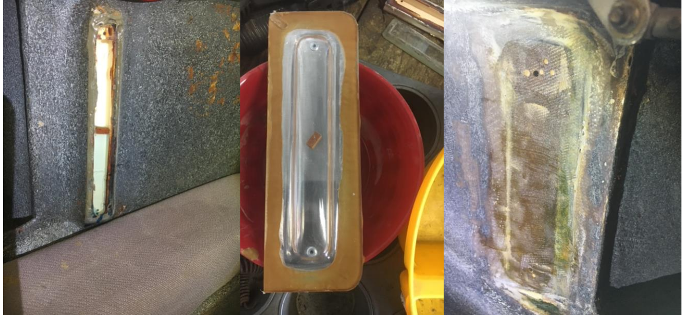
Figures: The leaky original sight glass, the new sight glass kit, the original hole filled in cabin.
