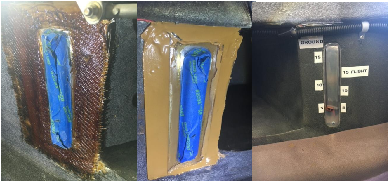
Figures: Fiberglass completed, filler completed, new site glass installed and calibrated.
