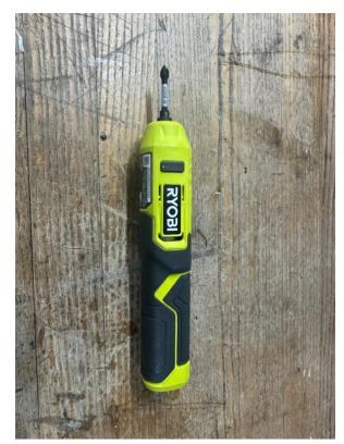
Electric screwdriver. This RYOBI screwdriver has a maximum torque perfect for AN-3 screws and is very compact. It certainly makes removing and reinstalling all the inspection ports a lot easier than with a normal screwdriver. I prefer this to other electric screwdrivers due to its compact size and low maximum torque.
