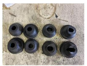
Engine Mounts: These parts sit in a harsh environment of heat and vibration along with absorbing thrust loads. The rubber components have a useful life of about 10 years and should also be inspected and swapped out on a regular basis. (Photo courtesy of Troy and Tracy Chaddon).
