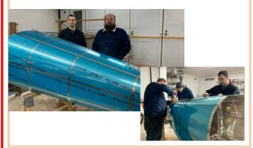
**January 12th** Tonight Mike Engseth, Tom Tolten, and John McPeak joined in to complete fitting the fiberglass fairings for the vertical stabilizer and rudder. They fit well.
