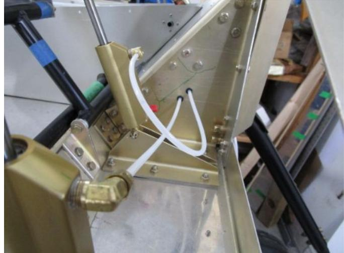
Copilot brake valve with lines from pilot side
