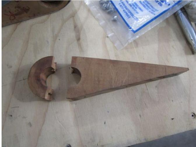
Not what you want to see when you open a flight control! So, out came the wood glue and clamps and 24 hours later the rib was ready to be re-installed and adjusted. Once it was reassembled we put it and the flaps back on the wing and re-installed the wing which leads to .....
