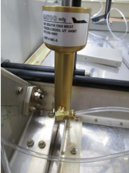
Pilot brake valve/reservoir with temp line
