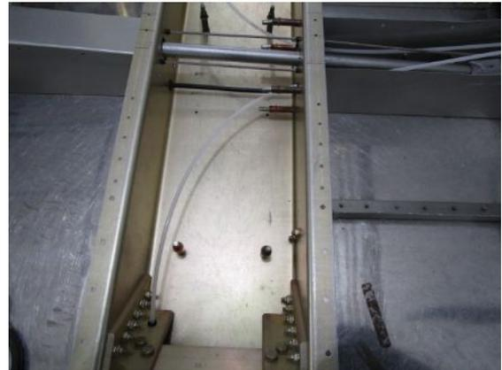
Right brake line running aft from tunnel through the main gear box and down to the gear strut and brake.
