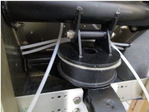
Brake lines passing through the nose gear box. The two unattached lines will be connected to the copilot actuators and run down to the brakes.
