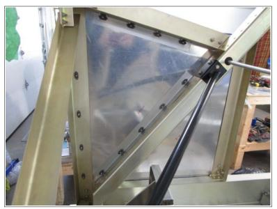
keep the skin tight on the frame. While the yoke would reach without issue, the dies were too thick to fit in line with the screw holes. After a bit of panic, I found some 0.063" aluminum, drilled it out to 3/16", then used 1/4" and 5/16" bits to counter sink the hole then used it in place of the female die on the inside of the L-bracket screw holes.
