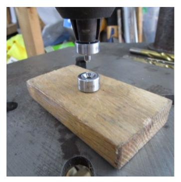
that is useless for anything else. After talking with the company engineer, I ordered some 0.032" sheet to replace the normal 0.016" skin, cut the skin on the left side back to a vertical stringer that the rudder controls are mounted on, and got to work drilling screw holes and dimpling skin. My trick with the drill press for dimpling came in handy again as I wanted one screw in the center or a diagonal frame piece to make sure there was no oil canning.
