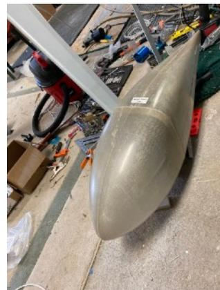
The cowling fitting was the most difficult so far. The top cowling was fit, but determined to have been cut too much at the bottom juncture and had to be replaced by the factory and fitted again - this time correctly. Also the canopy fiber glass fit around the front and rear had to be molded to fit. This was easier than anticipated.
