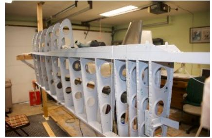
looked alike. Thank God for the numbering system of the parts by SPA. Measuring for square and level on the jig was a challenge. I am glad I had the factory build the main spars and fuel tanks as it would have increased my building time a few months.
