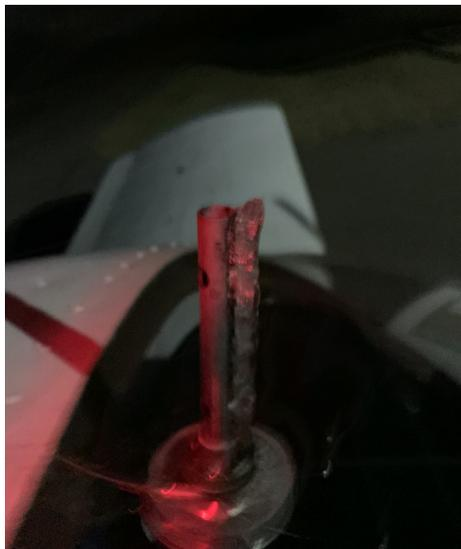
I took this picture while wearing my red headlamp I use when flying at night. There is about 1/4 inch of rime ice on the temperature probe. We were at 6,000 feet above the clouds and picked up the ice during the instrument approach
