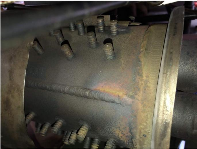
Example of crack in muffler (Image courtesy of Ben Showman)
