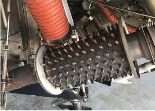
Muffler shroud removed
