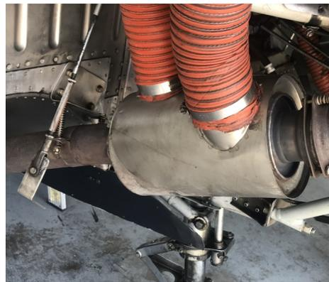
Example of a muffler shroud
