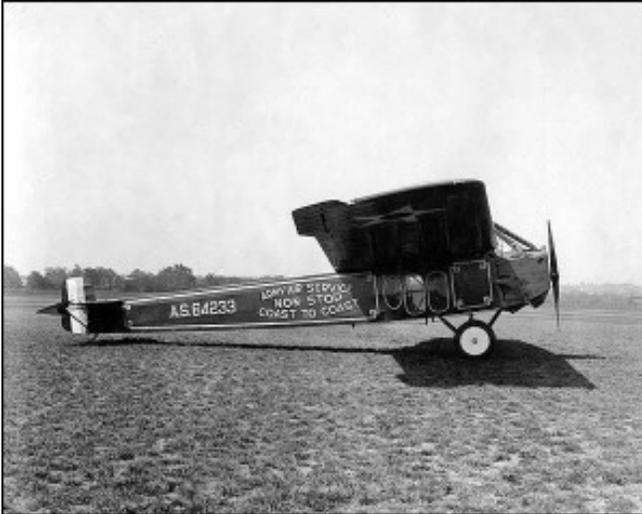
Having performed its notable feat, the big craft now rests in the Aircraft Building of the Smithsonian Institution in Washington. Its wingspread is 74 feet 10 inches; its length, 49 feet; and its height, 11 feet. The power-plant is a 400 H.P. Liberty engine. The old map of the United States showing the route followed by Macready and Kelly is still pasted in the fuselage.
