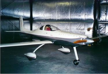
This is my project. It is a Silhouette. FAA signed it off in mid July (04). Power is via dual carburetor Rotax 447. Wingspan is 32'. Cruise is to be ~125 mph. It is hangared at Stevens Point. I am currently in the test phase. It has done a low pass over runway 21/03 at STE. I started the project in '93. After many starts and stops, it's finally finished.
