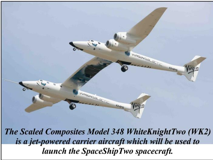
**The Scaled Composites Model 348 WhiteKnightTwo (WK2) is a jet-powered carrier aircraft which will be used to launch the SpaceShipTwo spacecraft.**
