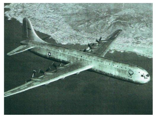
The 1947 press release from Consolidated Vultee Aircraft Corp. proclaimed this XC-99 transport-shown in flight off southern California- as "the worlds largest land plane." It was 182.5 feet long and 57.5 feet tall-longer and taller than its sister aircraft, the B-36, though they both had a 230-foot wingspan. The XC-99 had two levels of
