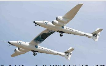
The Scaled Composites Model 348 WhiteKnightTwo (WK2) is a jet-powered carrier aircraft which will be used to launch the SpaceShipTwo spacecraft.
