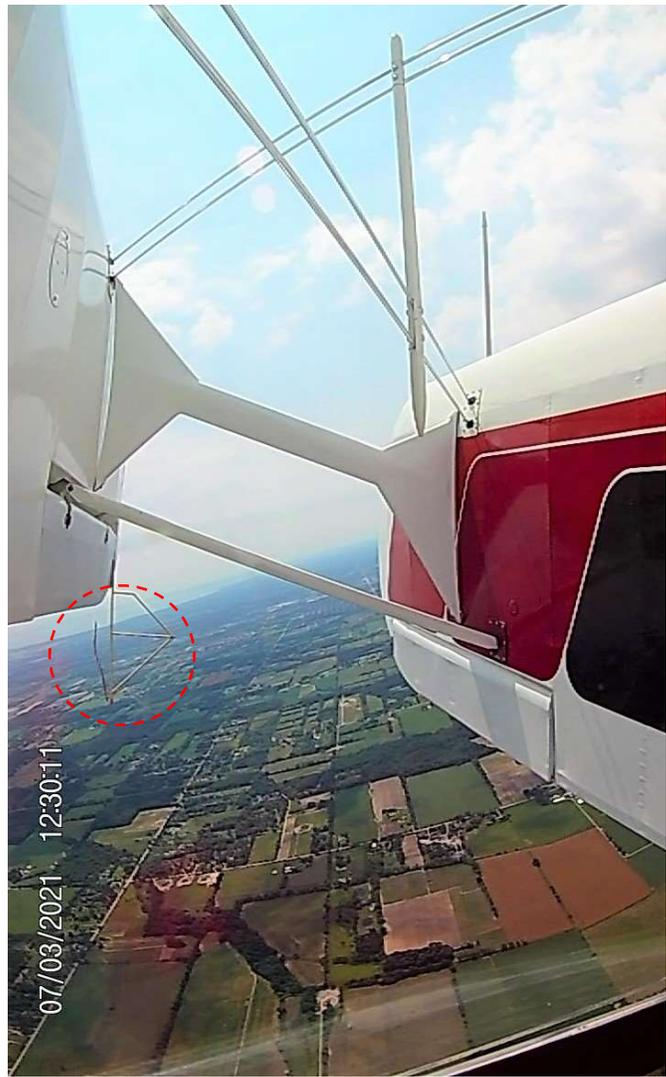
On the downline of a tail slide (string on sighting device point up)
