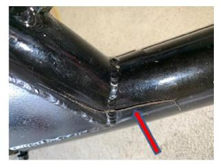
Gap opened near weld line when forcing stick to side with ailerons locked (clamped down)
