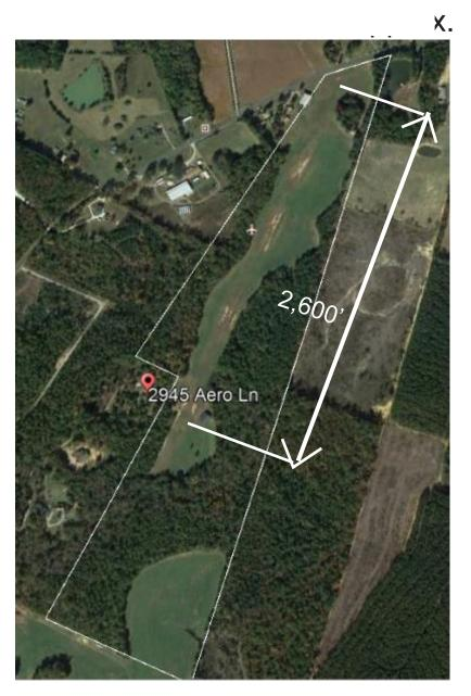
2,600' by 100' turf runway aligned 03 / 21 with additional 200' run off area, south end.
