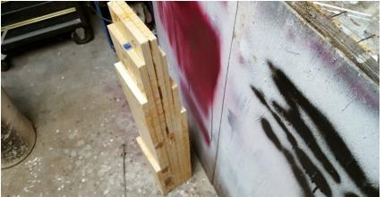
Once the glue has dried over night, the clamps can be removed. Then the outer profile or shape of the propeller is cut for each blade. It is very important to be extremely accurate with your lay out lines and cutting, since this cut shape will be your final propeller shape. Some minor changes can be made, but this shape is what drives the carving of the propeller.
