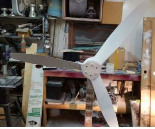
2 days after Flat side is glassed: Trailing edge of the prop wood is removed back about 3/8 of an inch before the shaped side of the prop is glassed. The glass is wrapped over the leading edge about 3/4 of an inch on the flat side of the blade. Once glass is stimpled out, Peel Ply is added to control the glass from moving and to give a good surface to work with during the finishing process.
