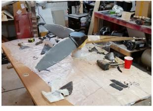
First Carbon layups. Flat side first. Layers of glass on each side of the blades. 18 Layers at the hub.
