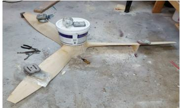
Fiberglass center hub with ¼ diameter carbon fiber spars wrap around the hub and down each blade. So far very happy with the progress for the prop. It has taken 6 nights of carving to get this far.
