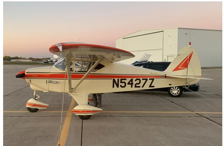
A little teaser pic on page two, and here's another shot of the Colt. As Piper was transitioning to the Cherokee as its primary 'family' airplane, the Colt was developed from the Tri-Pacer to fill the niche 'til the Cherokee was ready. Basically a two place Tri-Pacer, with 108 hp Lycoming engine and single door
