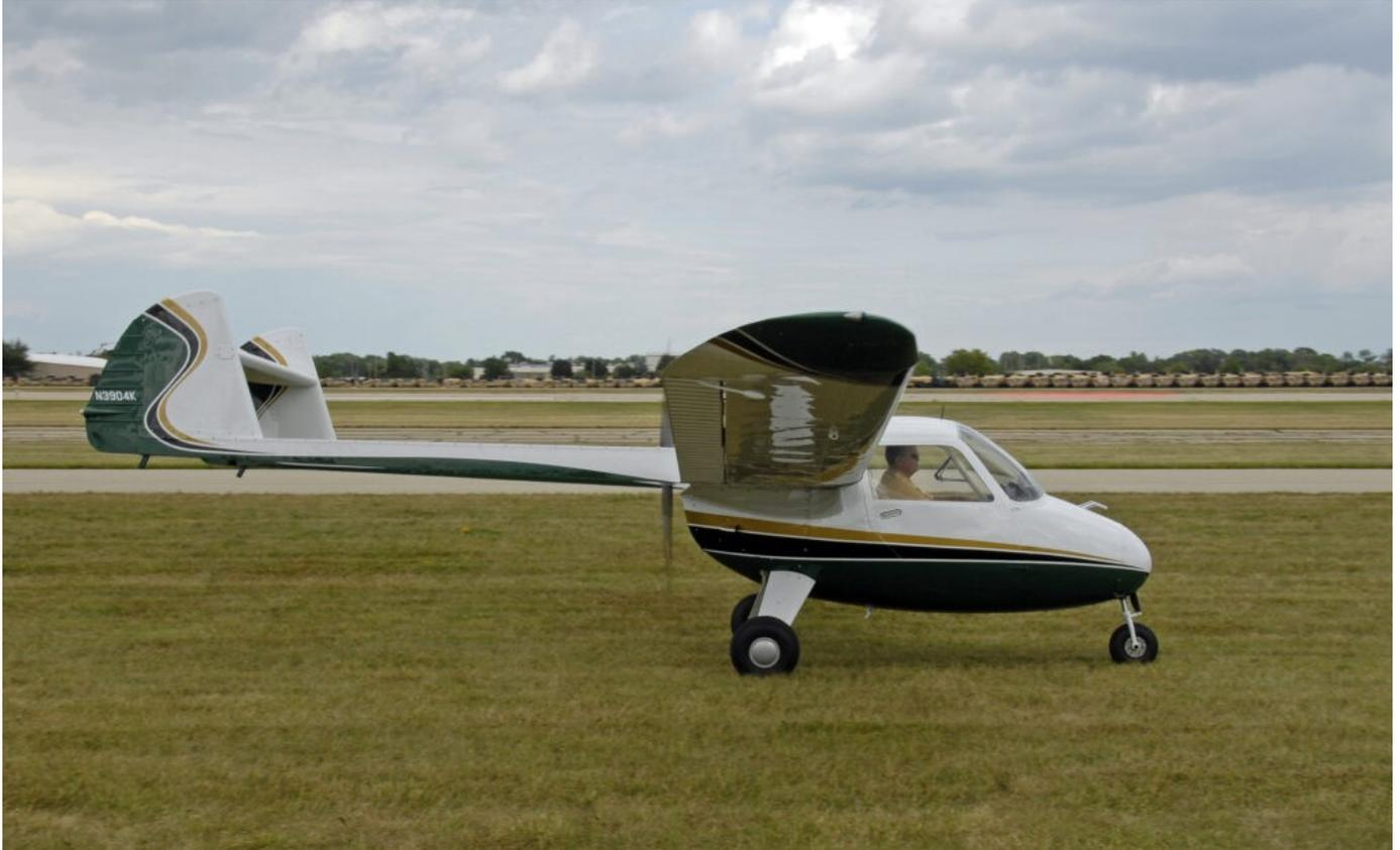
The AG-14 was built in 1950, there were 5 built with 4 remaining and registered. Powered by a Continental C-90 (90 hp), cruises at 110 mph, climb rate 630' fpm.
