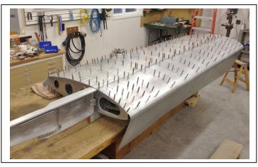
the skins in place, the wing is very straight and rigid. I have the wing turned over (thanks to Dave Swanson for being my "chief assistant wing flipper") and am fitting the leading edge to the underside of the wing. LOTS of hole drilling and clecoing!!
