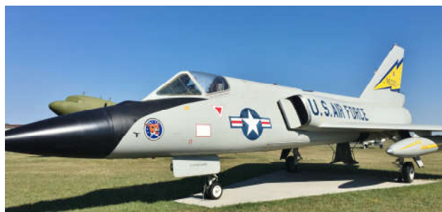
The F-106A (single seat) Delta Dart. We also had two of the F-106B (two seat) versions of this Mach 2+ aircraft.
