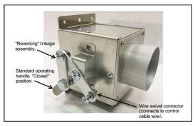
The addition of this device allows me to "pull" a knob on the instrument panel (the knob is one end of a wire which is connected to the reversing linkage) which then "pushes" the cabin heat box valve from its "Closed" to "Open" position. Vise versa when pushing the knob on the control cable to shut off the heat.
