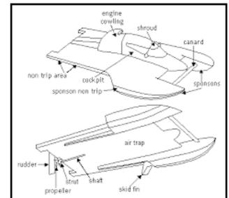
Notice the front where air enters the space under the bottom and is confined by the air-traps. They are called air-traps because as the hydro moves forward, air goes into this space and gets trapped there, causing a lift on the boat. I will explain how this works and what happens to the air trapped next.
