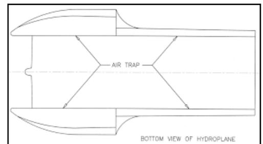
Air inlet size is the Width X (S.D. + H) so for a 35 inch wide bottom with 2 inch deep sponsons (S.D.), riding 1 inch high(H), the total intake area will be 105 square inches. The exit area will be the length of the afterplane (or air-trap length) times H. Say the afterplane is 65 inches, then the total exit area is 65 square inches when H is 1 inch (the exit area is 1/2 of 65 square inches on each side).
