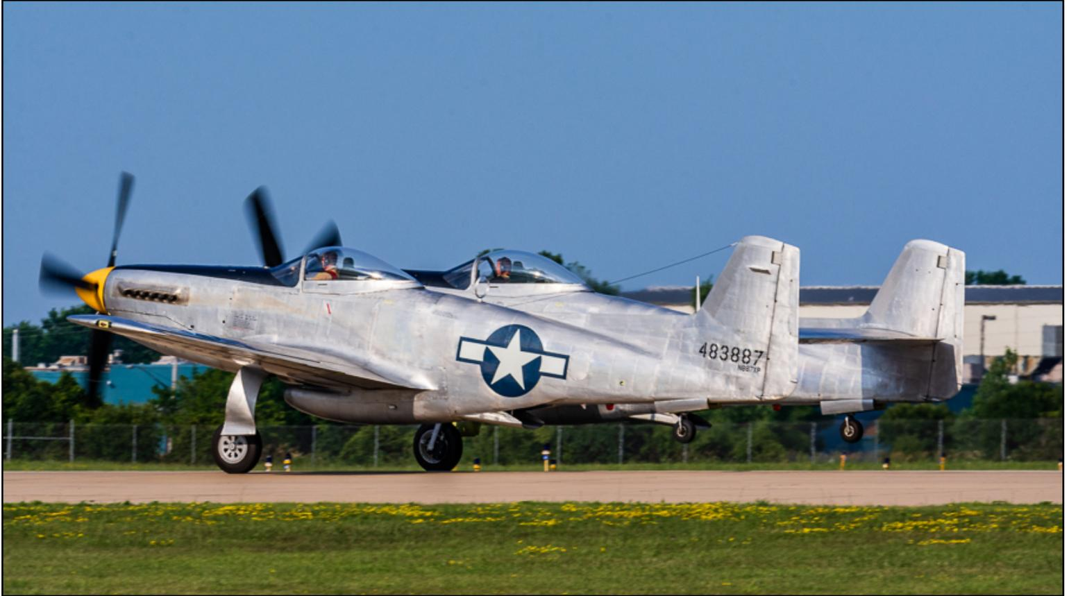
I will relate a couple details though, this airframe, the second prototype was first to actually fly in 1945, the design was intended for use as a long range escort for B-29 Super Fortress bombers in the Pacific. Its interesting to note that there are less than a half dozen components on the aircraft's airframe that are common with the P-51.
