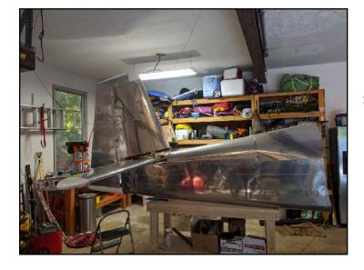
"Pictured at left are the completed empennage and tail cone for the project."
