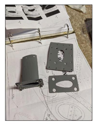
"These are parts of the Pitot mount assembly right after I primed them. This is a Gretz Pitot mount for a Garmin Pitot."
