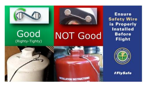
Failure to properly secure aircraft components can compromise powerplant and control system operation, leading to system and component failures. Properly secure aircraft components with safety wire, ensure that hardware locking mechanisms are properly installed on your aircraft, and check them often to confirm they are taut and ready for flight.
