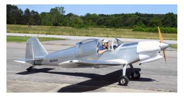
some roll issues, trying to make the left brake better, and some kind of charging glitch. Getting about 126 mph true airspeed with 3000 rpm. Haven't stalled it yet. -Ron
