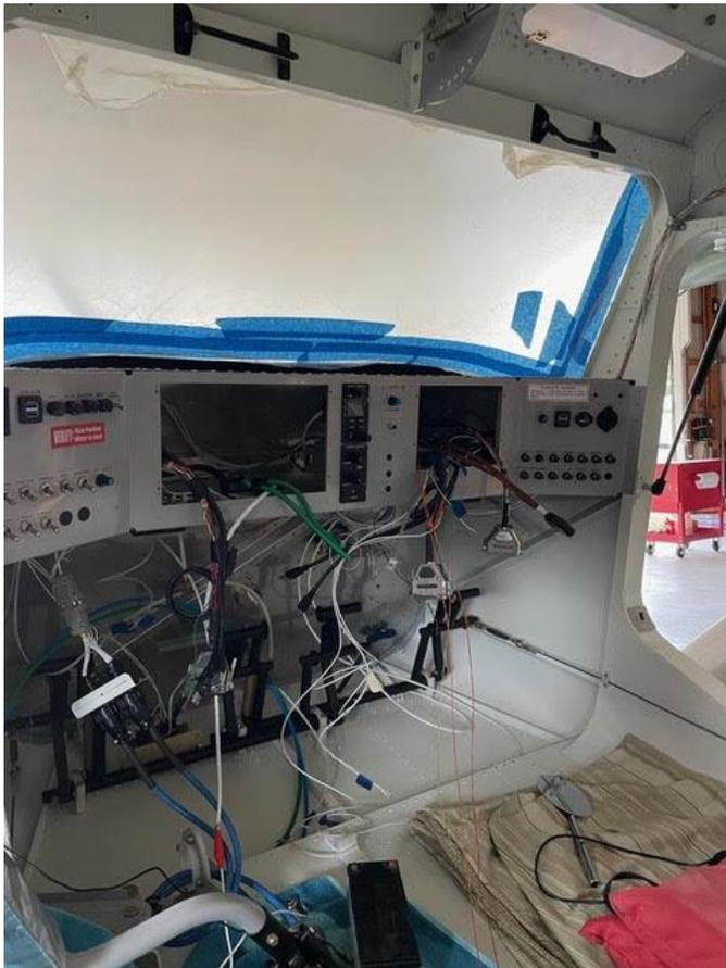
Paul's airframe is 99% complete. The engine is mounted. The panel is installed except for the two main glass panels. Those panels are out right now to allow access to everything behind the panel. The panel was completely wired up before installation.
