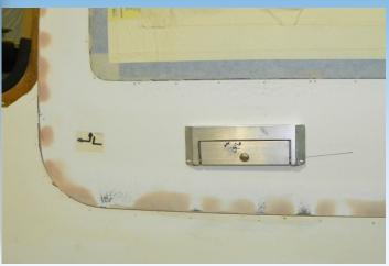
Pull, turn, lift. Interestingly, the handle shown here is heavier than the pin-and-cam latch mechanism it operates inside the door. But it all functions nicely together.
