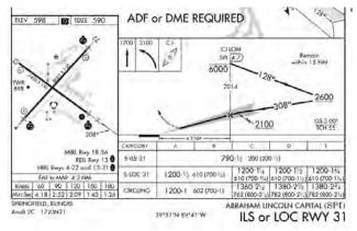
here you have 3 sections. The airport diagram is the same one from the Airport Facilities Directory /AF/D with the exception of that arrow pointing to 31. The arrow indicates how the approach is aligned with types of approaches might not be lined up with the runway at all. Consider an airport in a canyon.. you might have to fly to a localizer like device and then turn to the final approach. In our case the ILS brings us right down the centerline.
