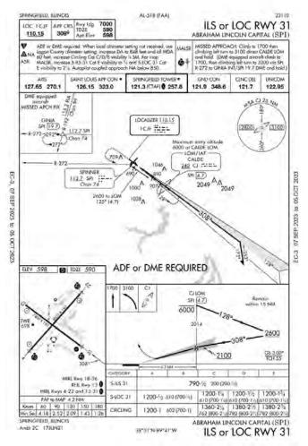
An ILS (Instrument Landing System) approach gives you both lateral and vertical guidance as it uses the localizer (aligned with the runway) and a glideslope (a constant 3ish\* path down to the runway).
