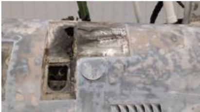
Fuselage Sections & a critical access panel hidden under two inches of plastic filler uncovered, reformed & repaired with hydraulic pressure and fresh skin by Dave Rudd, Zeke and others.
