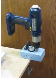
Using the same drill bit, I chucked the bit into my cordless drill and then returned the bit into it's hole in the block of wood. The theory is that the cordless drill is now square with the block.
