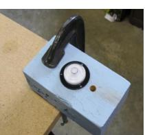
drilling a hole through the block. I then clamped that block of wood to my workbench, placing the second bubble level on the block. If the block is not level it needs to be shimmed to make it so.
