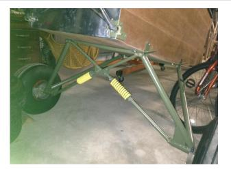
Completed gear showing die springs and wheels mounted.
