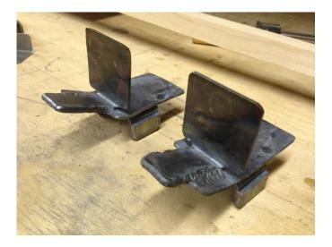
Lift strut/Landing gear fittings
