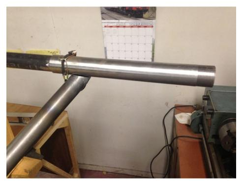
How the axle fit to the gear leg just prior to tack welding.
