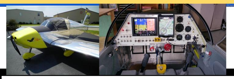
153 hrs TTF/E, Experimental Airworthiness issued 2013 Tri gear, dual controls, 16-gal main, 5-gal Aux, 21-gal total GPA 2276cc Dual Ignition VW Conversion, Prop: Prince P-Tip 54 X 44
