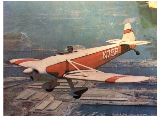
Joan Trefethen and her modified Stits Playboy circa 1960. Note the bubble canopy and squared-off shape of the fin and rudder. The gear legs are aluminum and the wings are modified from a Ryan PT22.
