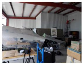
In this installment; I have included photos of the fuselage as it currently sits in my hangar, 7928-H, and the partially completed upper and lower wing, and tail surfaces that I am keeping in my home in order to-take advantage of a temperature controlled environment, to minimize warping and superfluous damage to the wooden structures, until ready for final covering and assembly. The big challenge now is the engine and its associated hardware.
