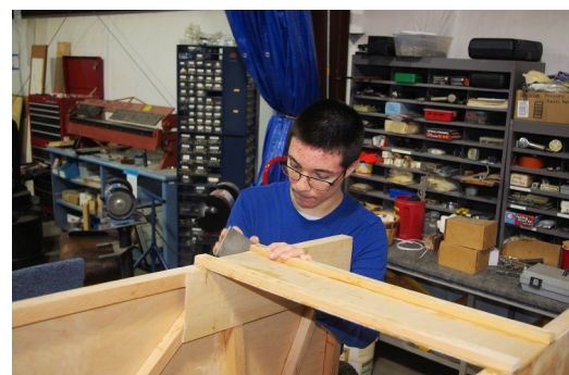
Paul's sanding the cross member flush with the fuselage side.
