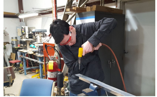
David Anders drilling on a fixture for building the aft fuselage.
