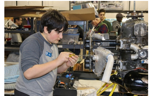
Max removing a valve cover on the Continental
