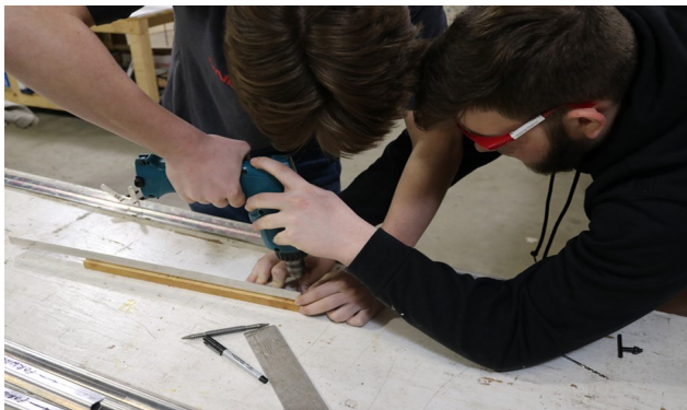
Jackson drilling a piece of the aft fuselage while Ben makes sure the drill is straight.
