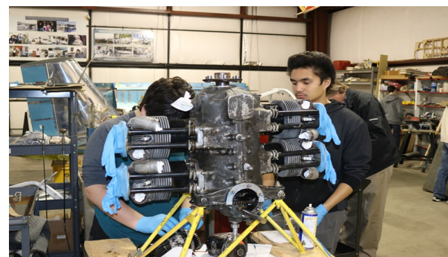
Max Kramer and Josh Wood are working on disassembling the Continental A65
