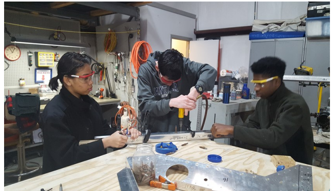
David Anders drilling on a fixture for building the aft fuselage.
