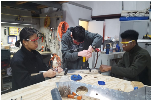
Moe, David and Learh doing some drilling on the right side cabin structure.
